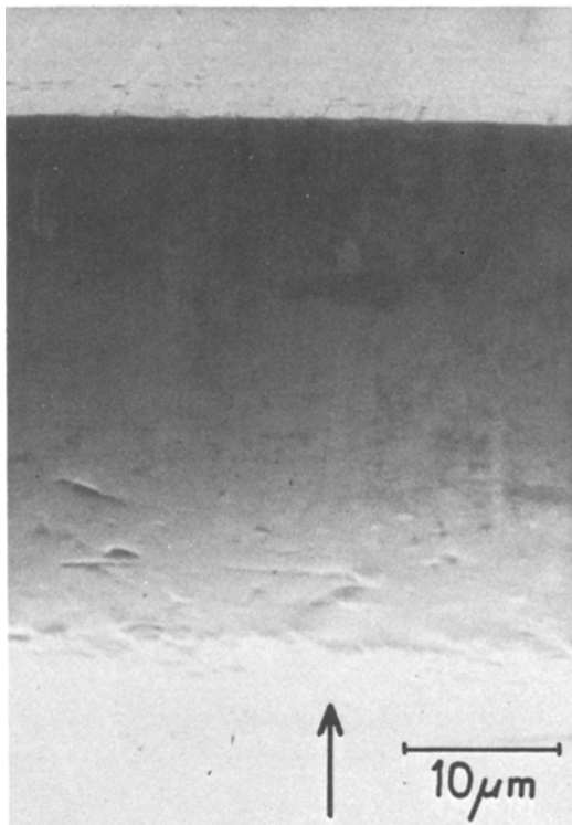
Figure 3 Edge of a "Schick Plus Platinum" razor blade after abrasion against SBR in nitrogen. The direction of rubber motion is indicated by the arrow.
